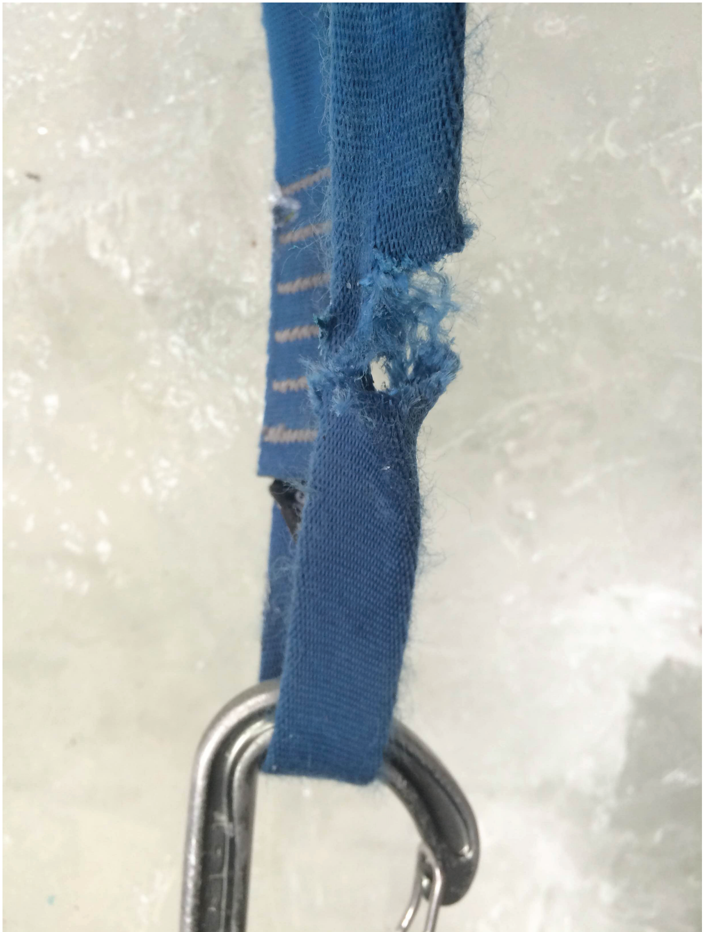
Enormous forces has been at work during the fall and almost completely ripped the nylon sling. Photo by Martin Skaar Oslund
