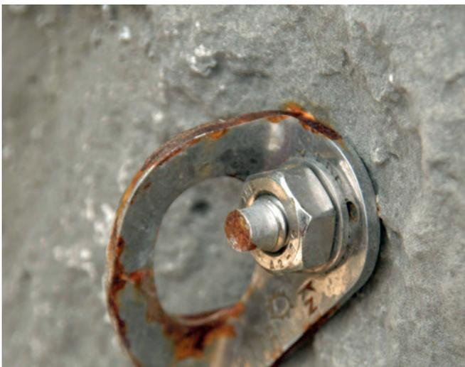
*Fig. 51 A bolt system incorrectly heat-treated during manufacture two days after setting in a subtropical climbing area by the sea.*
