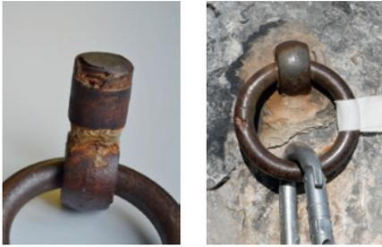
*Fig. 13 Second generation DAV ring bolts (CAUTION!). From the outside, this system is easily recognizable by the typical sealing compound that surrounds the anchors. Rust traces are often visible here when corrosion has started in inside. The outer diameter of these rings is 75 mm, the ring thickness is 12 mm.*
