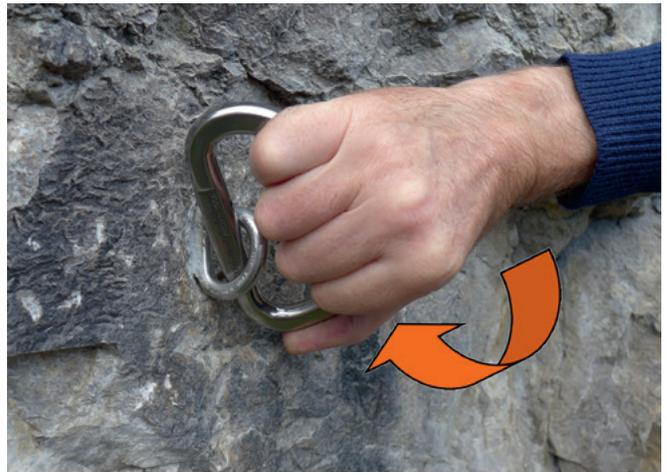
Fig. 31 Carabiner rotation test to check whether the bonding agent has set correctly. Attention: do not apply more torque with a larger lever. If more torque is used, a good bond may be destroyed under certain circumstances!
