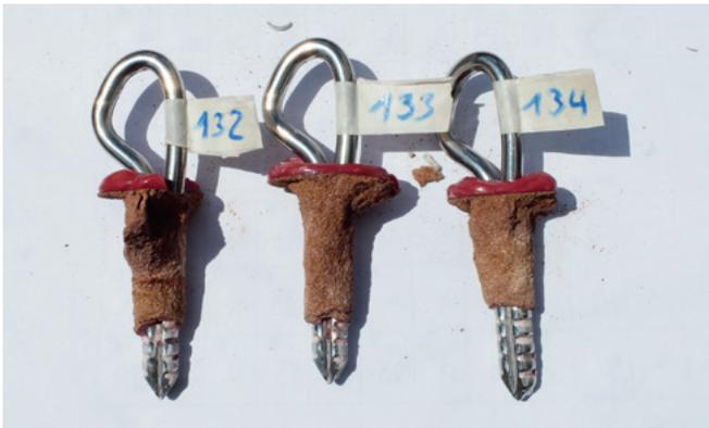
Fig. 39 During the pull-out tests in the red Main sandstone, the soft rock gave way. The rock around the bolt was pulled out of the wall like a cork.
