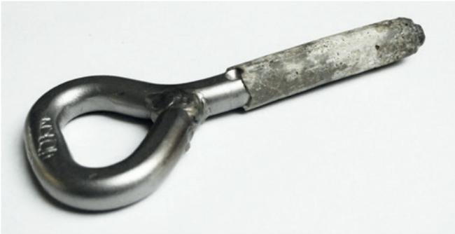
*Fig. 28 If the borehole is not cleaned, the bolt will only bond with the drilling dust, but not with the borehole wall. It can then be extracted along with the bonding agent at relatively low forces.*
