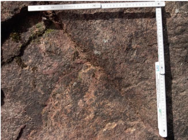
*Fig. 56 The rock in the lower area at the Swimming Pool Rock (a former quarry) is a slate-like porphyry. Due to the risk that the compressive effect of the heavy-duty anchors could have a detrimental effect on the slate-like structures of the porphyry here, the crag was equipped exclusively with glue-in bolts.*
