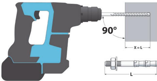
Fig. 45 The hole is drilled 90° to the rock surface and, in the case of the express anchor, at a depth corresponding to the anchor length or a few millimeters deeper.
