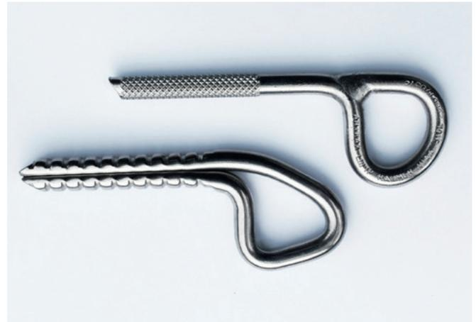
*Fig. 33 The glue-in bolt from the manufacturer Raumer (top single-axis, shaft length 80 mm, diameter 8 mm) was used for the pull-out tests of the glass bonding agent capsules, while the cartridge bonding agent was tested with the bolt from the manufacturer AustriAlpin (bottom double-axis, shaft length 75 mm, diameter 12 mm).*
