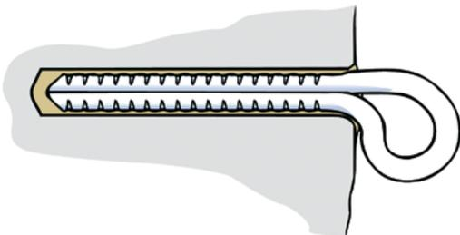
Fig. 3 In the case of glue-in bolts, the bonding agent (yellow) creates the „material or adhesive bond“ necessary for strength
