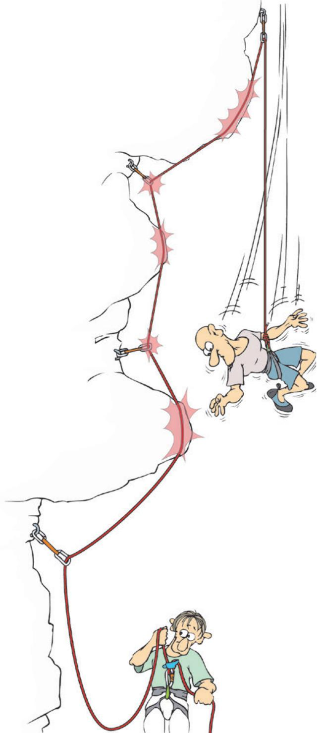
Fig. 72 Unfavorable positioning of the bolts creates unnecessary rope drag.
