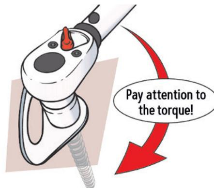
*Fig. 47 Even with screw anchors, the maximum torque must be adhered to according to the manufacturer's specifications.*
