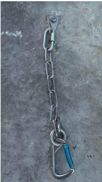
*Fig. 74 A cut-to-length anchor with two different types of bolts that can be adapted to the rock conditions.*
