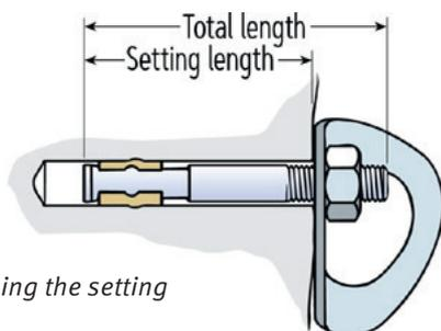
Fig. 6 Dimensioning the setting length of bolts
