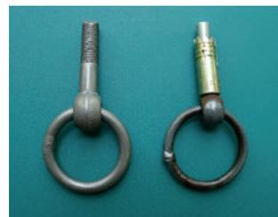
Fig. 12 Easy to confuse from the outside: on the left a glue-in, on the right an old self-drilling ring anchor. In the case of self-drilling anchors, the hole must be sealed to prevent the ingress of water and the resulting corrosion. The sealant looks like bonding agent from the outside and hides the drill bit, making the problem invisible ...
