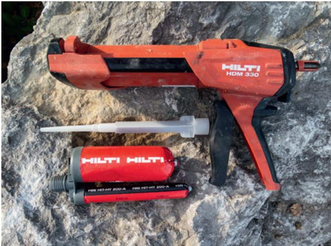
Fig. 26 Cartridge bonding agent: Bonding agent, squeeze gun and mixing nozzle must match!
