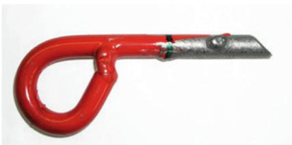
*Fig. 15 Attention! The so-called “Sigibolt” is a non-standard, glue-in bolt, a “home-made” brand, which was frequently used in the Hochkönig area, in the Dachstein and Tennen mountains and in the Gesäuse until about 2006. At first sight, this type of bolt looks confidence inspiring, but due to design-related defects, its strength must be considered similar to the strength of a normal piton („hammered in piton“)!*
