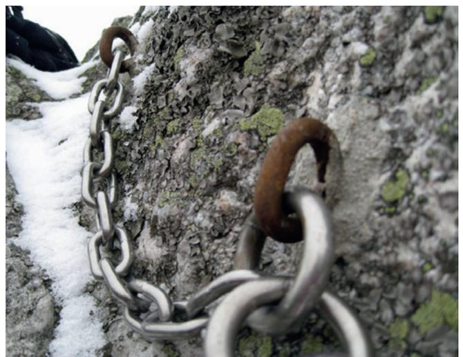
*Fig. 50a/b An anchor chain as manufactured (left) and after a few months on the rock (right). Rings and chain links were made of a corrosion-resistant steel with about 18% chromium content, the bolts shown were accidentally made of a normal mild steel.*
