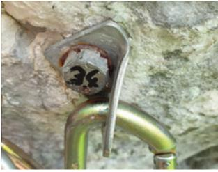
Fig. 20 Self-drilling bolt from the DAV safety research pull-out tests
