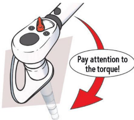
*Fig. 47 For wedge anchors, it is essential to observe the maximum torque (between 25 and 45 Nm for M10 according to manufacturer's specifications). The anchor should protrude slightly above the screw (approx. 3-5 mm) after reaching the tightening torque.*
