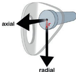
Fig. 5 Pulling directions for bolts and rock anchors
