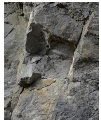
Fig. 70c After the pull-out test - the rock broke at 6 kN, far below the standard requirement for radial load of 25 kN.
