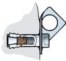
Fig. 9 Contact corrosion in the cavity of a self-drilling bolt
