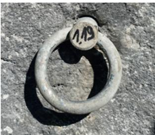
Fig. 24 Mammut ring in the DAV safety research pull-out tests
