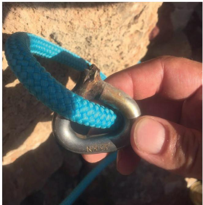
Fig. 53 Bolt fracture in marine environment. The steel used was not able to withstand the corrosive influences and broke under simple rappelling loads.
