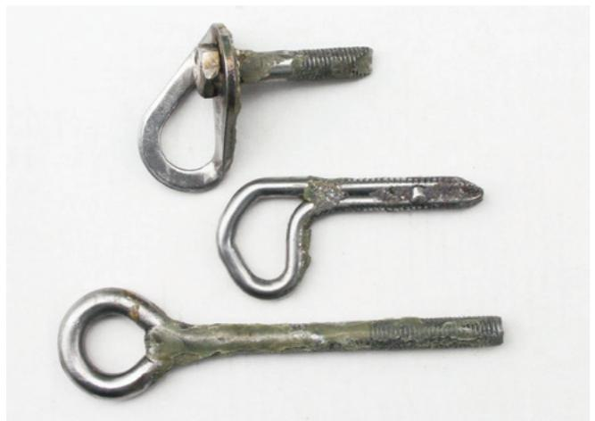
Fig. 32 If good bolts are set in solid rock with the right bonding agent, then they are reliable anchors. Improperly installed glue-in bolts are a life-threatening trap. Climbing was done on the bolts shown here—they could be pulled out by hand! A final inspection would have revealed the danger sooner!
