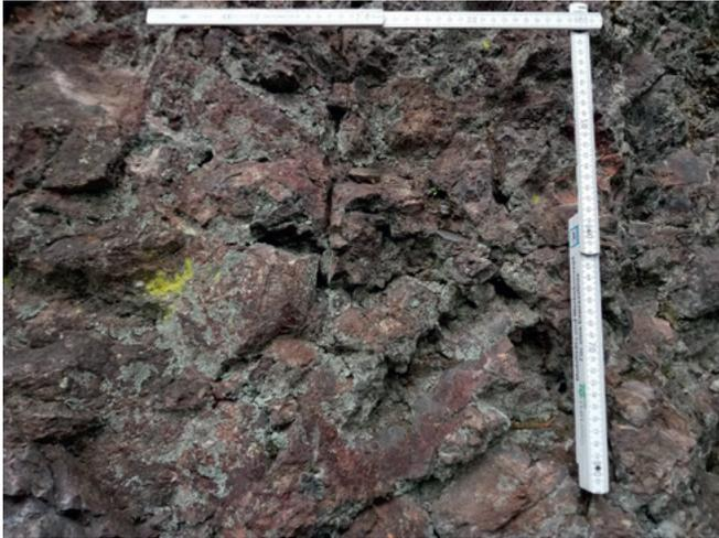
*Fig. 55 The finely structured porphyry at Lägerfelsen in the Triberg district is hard, but cavities are repeatedly encountered during drilling. That is why it makes sense to use glue-in bolts there in particular. The cavities can be filled with cartridge bonding agent. Glass bonding agent capsules are not suitable here because of the cavities.*
