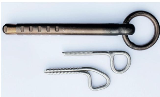
Fig. 40 Dimensions of glue-in bolts: above, a special bolt for the soft sandstone in the Elbe Sandstone Mountains; below, the bolt models for solid rock used for the DAV Safety Research tests
