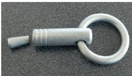
Fig. 11 Ring bolt expansion anchors without self-drilling bit – if the hole is drilled too deeply, the ring will be in contact with the rock before the cone at the bottom of the hole has expanded the anchor enough to sufficiently withstand axial pull
