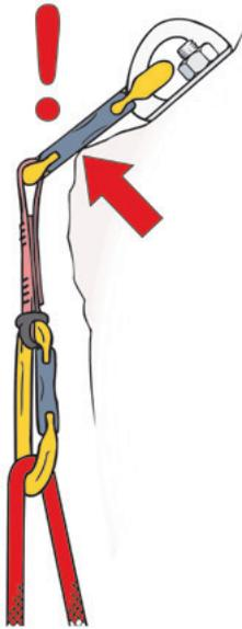
Fig. 71 This poorly placed bolt induces a buckling load on the carabiner.
