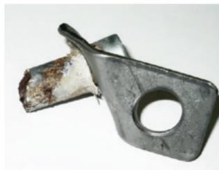
Fig. 10 This self-drilling bolt snapped during a sport climbing fall
