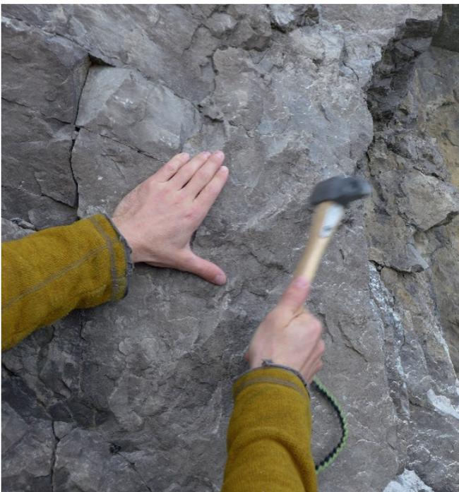
Fig. 70a Important: before drilling, the rock is tapped. The sound reveals where the rock is solid and without cavities. Only here can a bolt be reliable. If you feel the vibrations of the hammer blows in the hand placed on the rock surface, the rock is not solid at this point.
