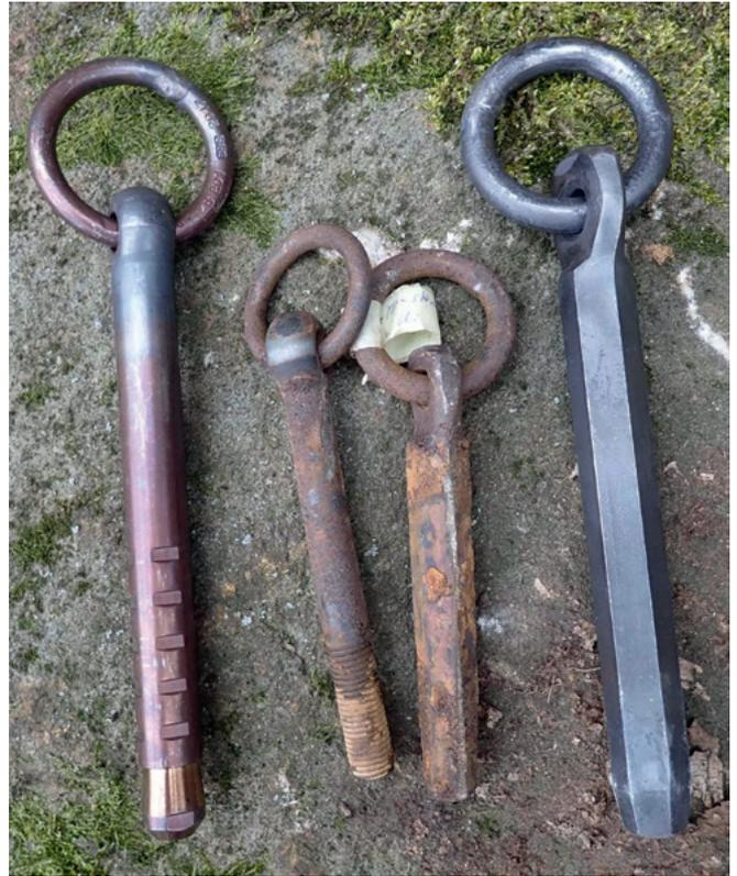
*Fig. 65 On the left a modern Elbe stainless steel ring, on the right a KTA iron ring, in between two undersized and therefore removed old rings. Photo: Wido Woicik*
