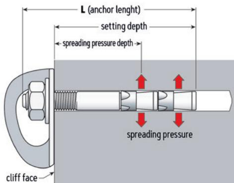
Fig. 48 Wedge bolts with double cones apply the expansion pressure to the rock in two places, but closer to the rock surface. The spreading pressure depth is significantly shorter than the anchor length. With an 85 mm long anchor of this design, the first expansion pressure acts about 40 mm below the rock surface.
