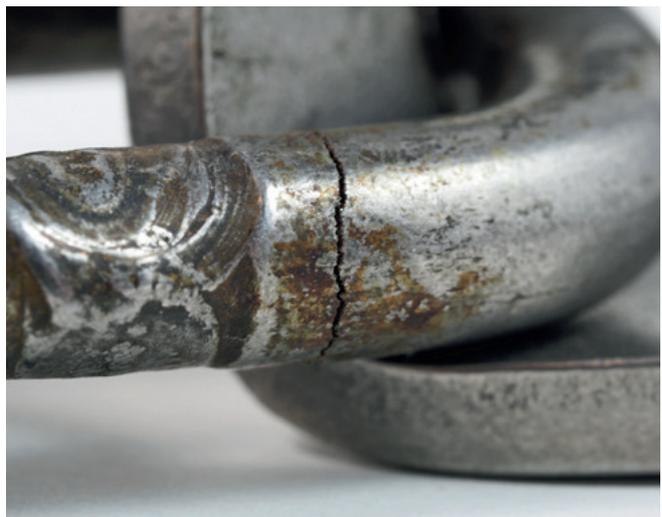
*Fig. 52 A crack caused by intergranular corrosion in the heat-affected zone of the welded joint of a chain link of an anchor..*
