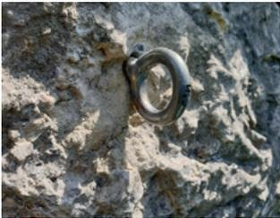
Fig. 21 Eye bolt from the DAV safety research pull-out tests
