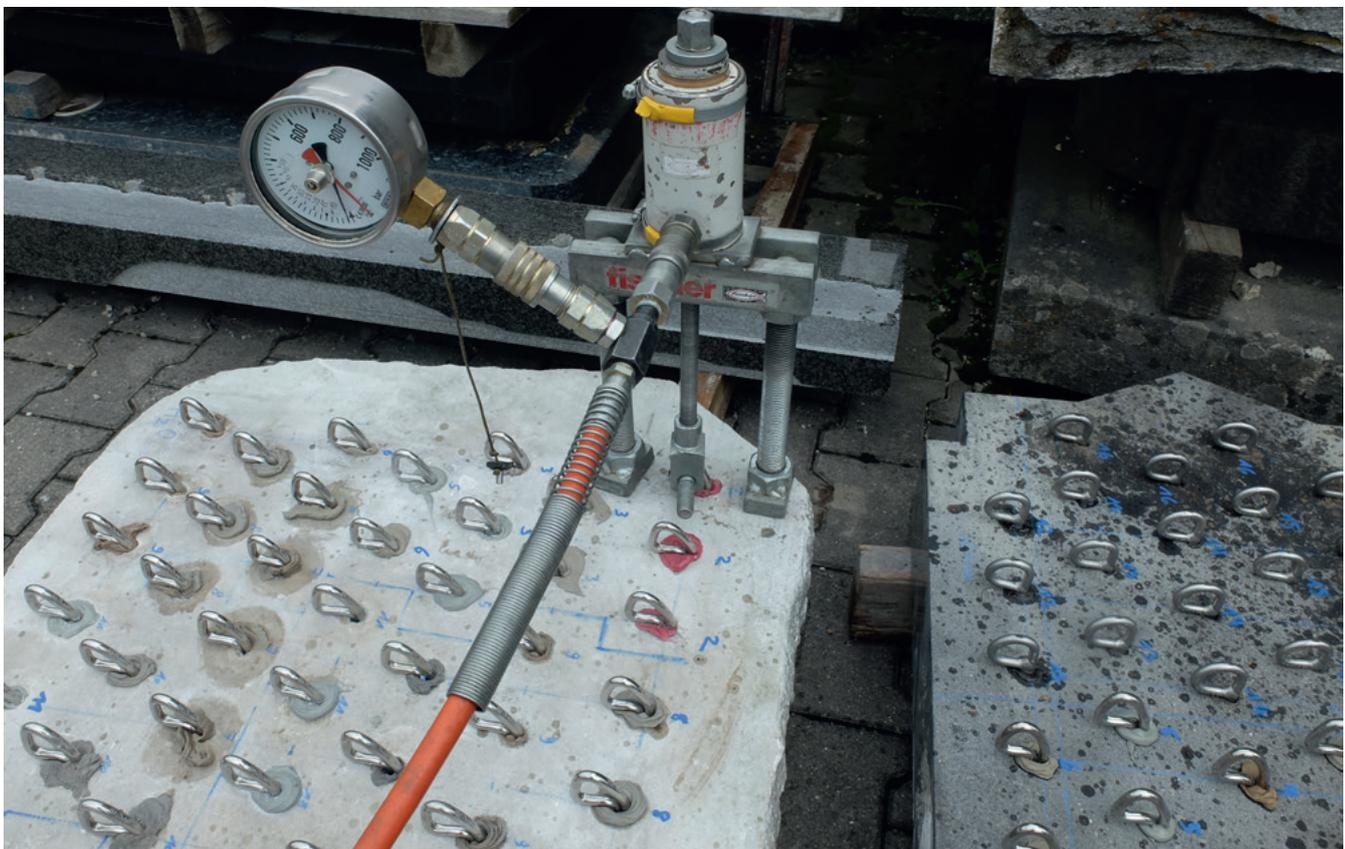
Fig. 34 Axial pull-out tests: left limestone, right granite.
