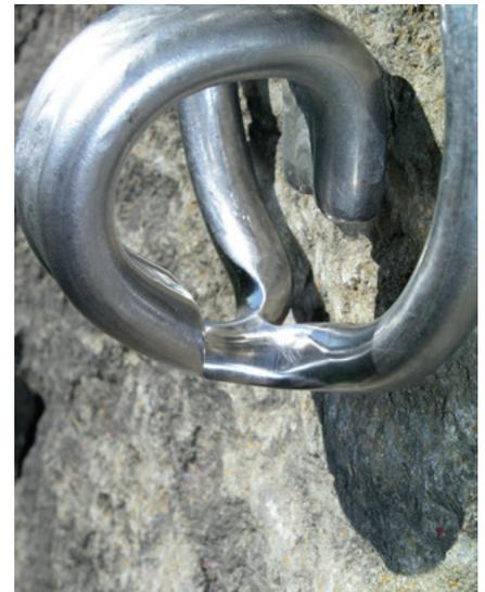
*Fig. 73 Example of an anchor abraded by topropes.*
