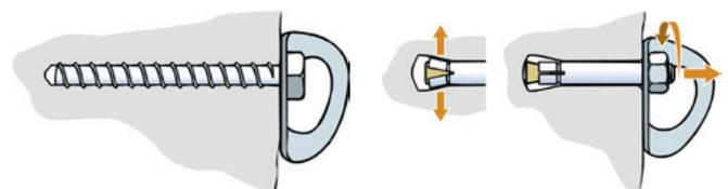
Fig. 4c Sleeve anchor
