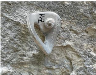
Fig. 23 Drop-in bolt with expansion cone in DAV safety research pull-out tests
