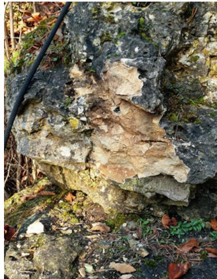
Fig. 19 Glue-in bolt from the bolt study with too little distance to the left (crack) and below to the edge. At a 6.8 kN radial load, the bolt pulled out together with the rock.
