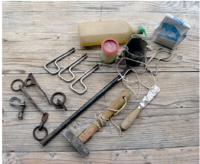
*Fig. 16 The original equipment with which Oskar Bühler installed his bolts. Photo: Christl Gensthaller (née Bühler).*
